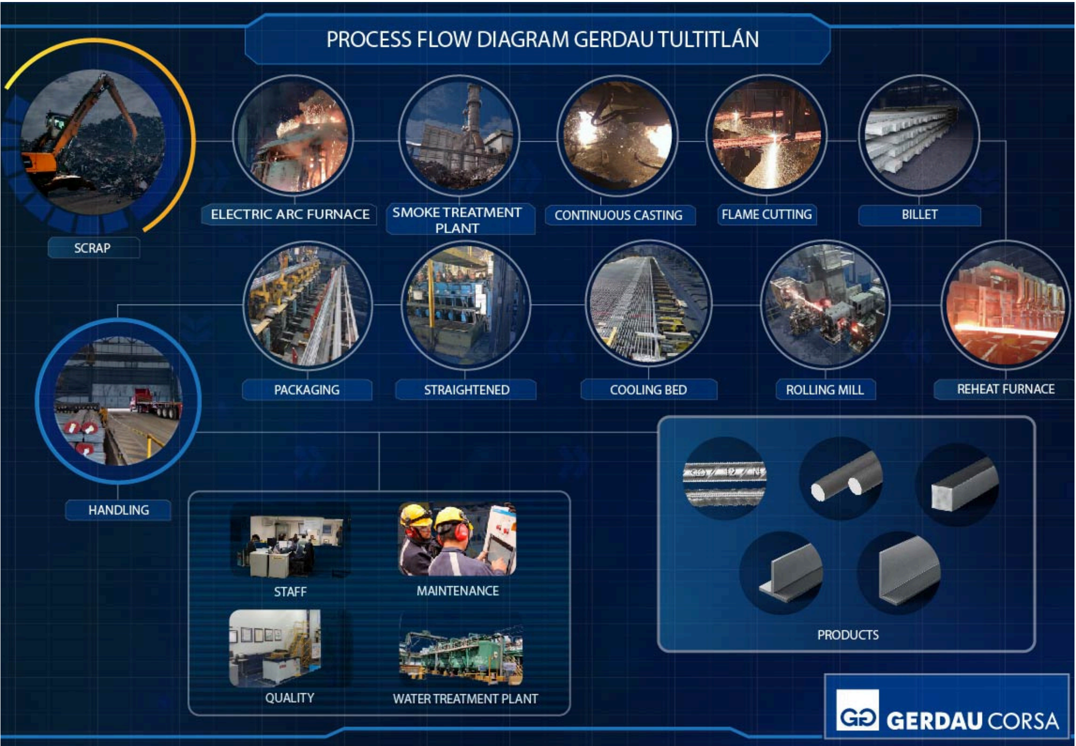
Figure. 2. Flow diagram of Steel rebar manufactured from steel scrap.
