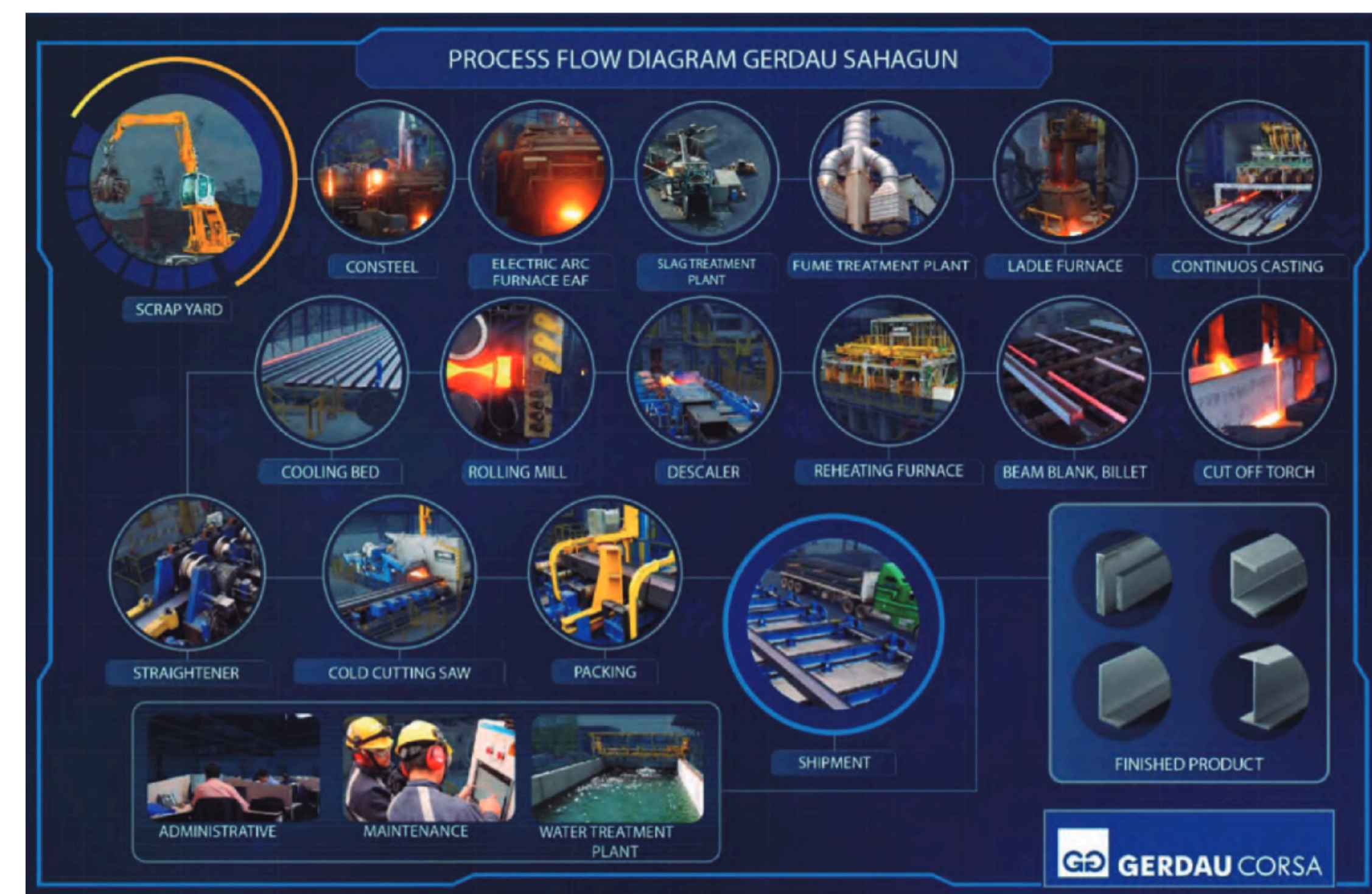
Figure. 2. Flow diagram of Hot rolled structural shapes manufactured from Hot rolled structural shapes.
