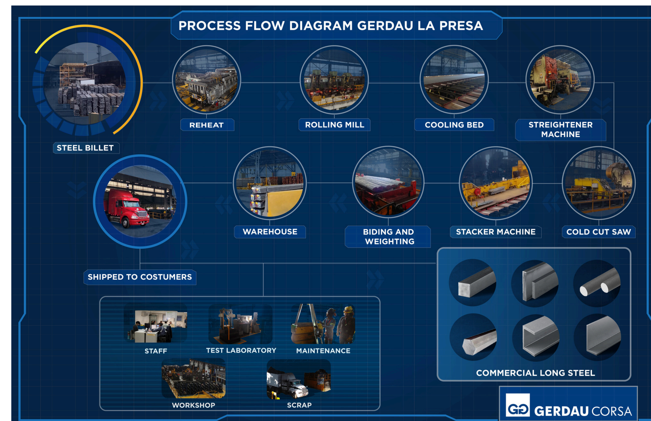
Figure. 1. Flow diagram of Commercial long steel hot-rolled manufactured from steel scrap.
