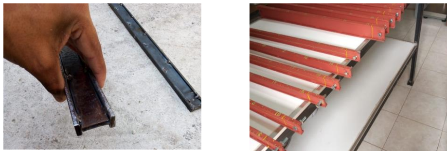
Fig. 2. Manufacture of piles to scale
